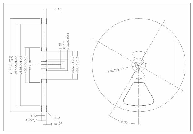
(2) Dimension of tape(Material: PS Conductive, 10E4~5Ω)
