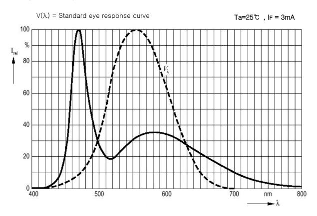
Fig.6 Radiation Characteristic
